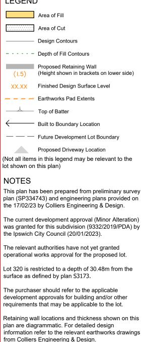
All fill shall be placed and compacted in a controlled manner under Level 1 supervision and certification in accordance with AS3798-2007.
