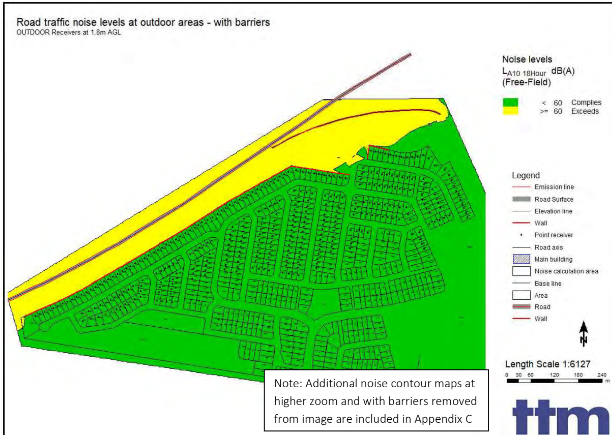
Figure 5: Predicted Road Traffic Noise Levels Compared to SDAP Outdoor Criteria (Cunningham Highway) – With Proposed Acoustic Barriers
